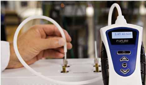
Figure 4: Probe connected to a GC gas outlet.
