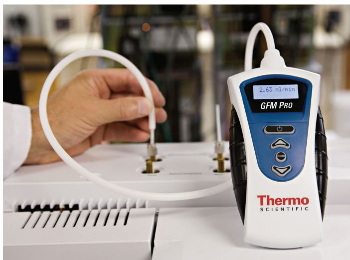
Figure 4. Probe connected to a GC gas outlet.
