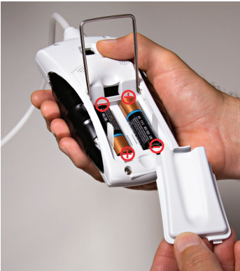
Figure 3. Insert the batteries as marked.
