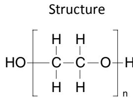
InertCap Pure-WAX is a high polar column bonded polyethylene glycol. Based on newly developed inner treatment technology, InertCap Pure-WAX achieves the highest inertness among the market available columns. InertCap Pure-WAX is a optimal column for analyses of acidic compounds and basic compounds that commercially available WAX columns were not capable of analyzing.
