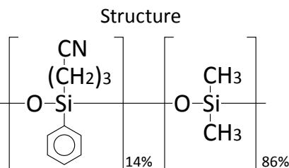
InertCap 1701MS is a medium polar column incorporating with 14 % cyanopropylphenyl and 86 % dimethylpolysiloxane, designed for GC/MS. Containing cyano groups as InertCap 1301, InertCap 1701MS has a stronger polarity than InertCap 25. It is suitable for pesticides screening analyses.
