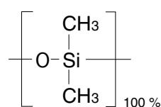
InertCap 1HT is a non-polar high-temperature column bonded with 100% dimethylpolysiloxane. Compounds elute in order of increasing boiling point. InertCap 1HT is specially processed for operation up to 400 °C with a high temperature polyimide coated fused silica tubing.
