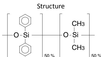
InertCap 17MS is a medium polar column bonded with 50 % diphenyl - 50 % dimethylpolysiloxane, designed for GC/MS.
