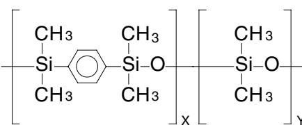
InertCap 5MS/Sil is a low polar column bonded with 5 % diphenyl (equiv.) – 95 % dimethylpolysilphenylene siloxane. Designed for GC/MS, InertCap 5MS/Sil achieves the higher heat resistance and lower bleeding by arylene technology. In addition to our basic performance and quality inspection, pesticide mixture sample is analyzed for the further rigorous inspection for each lot to guarantee the product reliability.
