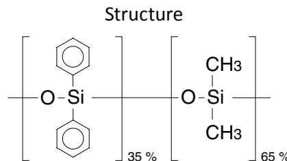
InertCap 35 is a medium polar column bonded with 35 % diphenyl - 65 % dimethylpolysiloxane. With a stronger polarity than InertCap 25, InertCap 35 also shows high separation efficiency for the analyses of semi volatile compounds and solvents.
