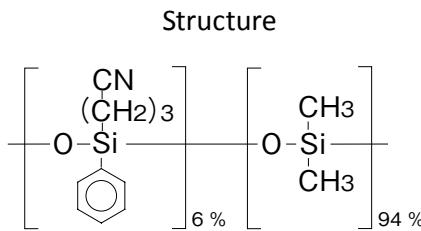
InertCap 624 is a medium polar column bonded with 6 % cyanopropylphenyl and 94 % dimethylpolysiloxane designed for VOC analysis. InertCap 624 is optimal for the analysis of “acetaldehyde and methanol in ethanol” defined in the Japanese Pharmacopoeia Fifteenth Edition.
