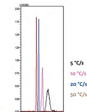
Influence of Cryotrap heating rate for Vinylchloride (M/Z = 62)
