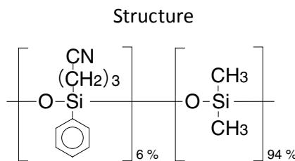
InertCap 624MS is medium polar column bonded with 6 % cyanopropylphenyl and 94 % dimethylpolysiloxane. The structure is the same as InertCap 624, designed for low bleed, stable batch control and highest inertness.
