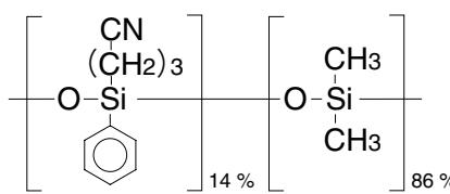
InertCap 1701 is a medium polar column bonded with 14 % cyanopropylphenyl and 86 % dimethylpolysiloxane. Containing cyano groups as InertCap 1301 InertCap 1701 has a stronger polarity than InertCap 25, InertCap 1701 is suitable for pesticides screening analyses.
