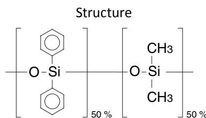
InertCap 17 is a medium polar column bonded with 50 % diphenyl - 50 % dimethylpolysiloxane. With stronger polarity than InertCap 35, InertCap 17 also shows high separation efficiency for general and pesticides analyses.
