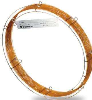
InertCap Fast GC is a column of I.D. 0.18 mm. Maintaining separation ability, InertCap Fast GC achieves fast analyses and best productivity with your existing GC instruments.
