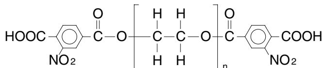
InertCap FFAP is a high polar column bonded nitroterephthalic acid modified polyethylene glycol. As the liquid phase shows acidity, it is possible to analyze volatile fatty acids without a derivatization. InertCap FFAP is optimal for the analyses of acidic compounds.
