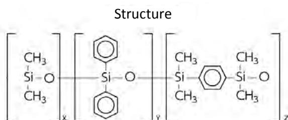
InertCap 35 is a medium polar column bonded with 35 % diphenyl - 65 % dimethylpolysiloxane. With a stronger polarity than InertCap 25, InertCap 35 also shows high separation efficiency for the analyses of semi volatile compounds and solvents. By increasing the heat resistance of the liquid phase, the maximum operating temperature of 360 °C can be achieved.
