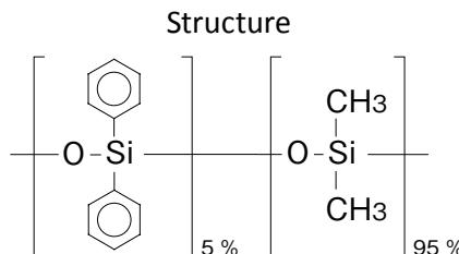
InertCap 5MS, in which liquid phase chemically bonded with 5% diphenyl-95% dimethylpolysiloxane, is a low-polarity column designed for GC/MS analysis with top level of inertness and low bleed.
