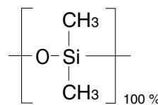
InertCap 1MS is a non-polar column bonded with 100 % Dimethylpolysiloxane. Samples elute in order of low boiling points. Designed for GC/MS, InertCap 1MS realizes the world highest inertness and ultra low bleed.
