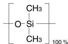
InertCap 1 is a non-polar column bonded with 100 % dimethylpolysiloxane. Compounds elute in order of increasing boiling point. InertCap 1 has broad utility and can be used for a variety of general analyses.
