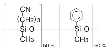
InertCap 225 is a medium polar column bonded with 50 % cyanopropylmethyl and 50 % phenylmethylpolysiloxane. Cyano group in the stationary phase includes triple bond and retains compounds stronger in accordance with the increase of the number of unsaturated bond by their dipole/dipole interactions. For that reasons InertCap 225 shows high separation efficiency for analyses of geometrical isomers.
