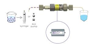
The sample matrix will be sent to waste while the target is analyte retained within the trap. The target analyte is now able to be eluted in a small volume of stronger solvent.
