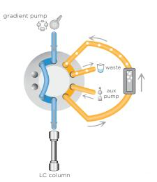
The anion exchange trap will have a finite capacity for SDS and must be regenerated before that capacity is exceeded.
