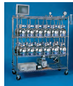
Figure 10: User-designed system for cleaning 24 six-liter canisters.
