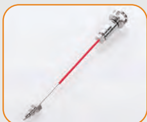
Compatible w/MODEL: 1260 CTS-21277 OEM G1367-87012 Needle Seat, 0.12mm ID, 0.8mm OD, PEEK™, 600 bar
