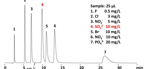
IC SI-36 4D uses potassium hydroxide aqueous solution for the analysis of anions.
