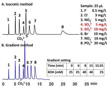
Column: Shodex IC SI-36 4D (4.0 mmI.D. x 150 mm)
