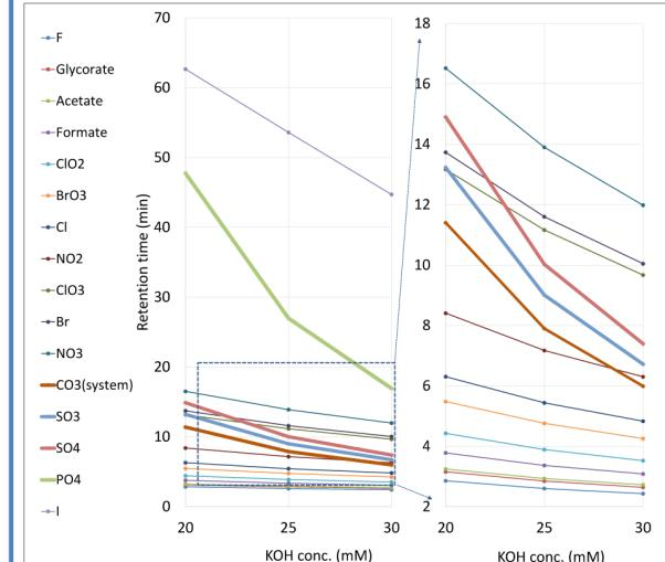
Column : Shodex IC SI-36 4D (4.0 mm I.D. x 150 mm)
