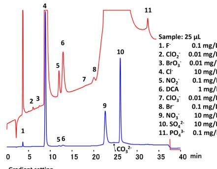
Column: Shodex IC SI-36 4D (4.0 mmI.D. x 150 mm)
