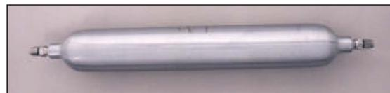
CHROMSPEC's layered bed, multi-purpose trap is designed to remove oxygen, moisture, hydrocarbons and carbon dioxide from gas streams. This 750cc unit will take the place of three separate traps, simplifying installation and reducing the number of potential leak sites that contribute to the aspiration of contaminants into the system. End fittings are stainless steel Swagelok™ fitted with 40 micron stainless steel frits.
