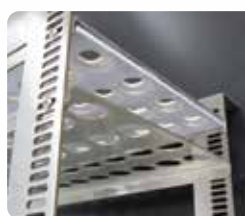
(Fig. 3) Tray guide attachment to assembly of tray sides and top
