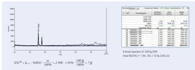
Also, ensuring the superior sensitivity of the YL6900 GC/MS, its S/N ratio is higher than 1500:1 by 1 pg injection of OFN in scan mode.
