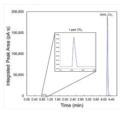
The Jetanizer's higher catalytic activity, as compared to nickel catalysts, allows for a larger linear dynamic range. Here, a linear dynamic response to  $\mathrm{CO}_2$  is depicted, from ppm to 100% concentrations.
