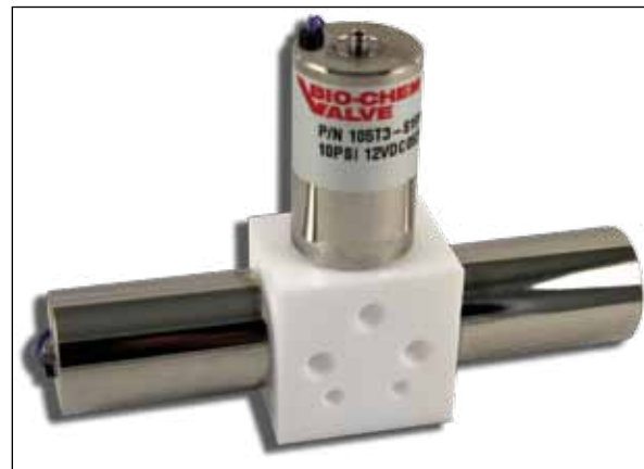
105T3 Flow Selection Valve (3 inlet ports, 0.125" orifice, PTFE body, PTFE diaphragm)
