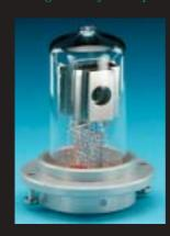
Deuterium lamps produce a plasma ball approximately 0.5mm in diameter. Disturbing the filaments by tenths of a millimeter will wreck the alignment of your bulb.
