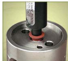
3. Then, the seal is pressed into the pump head seal cavity using the insertion support.
