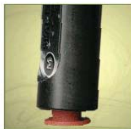
2. The piston seal is formed by pressing the tool onto the seal jacket.
