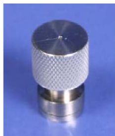
Stainless Steel TCLP Fitting with Replaceable Septum
