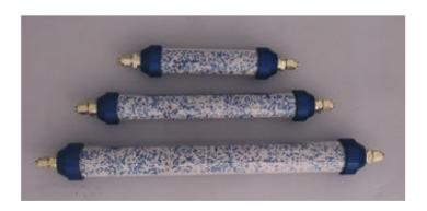
CHROMSPEC™ moisture traps utilize polycarbonate bodies, more inert and resistant to infusion than the acrylic used by other manufacturers. These traps are refillable and available in three sizes with three different adsorbent combinations. The ends are provided with Swagelok™ tube fittings. Each end fitting includes a 40 micron sintered stainless steel frit. Maximum pressure is 125 psi.
