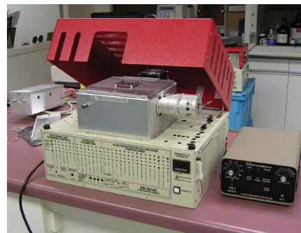
SRI GC with pulse discharge detector for low PPB work
