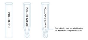
Limited volume inserts are an economical solution when there is a limited amount of sample and injection is done using an autosampler. Most autosamplers have a set depth that the injection needle can go into the vial without bottoming out. Inserts increase the sample depth within the vial even if there is a very minute volume of sample available.
