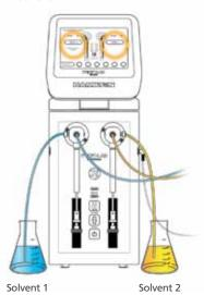
**Step 2.** Trigger the hand probe to fill the left and right syringes with Solvents 1 and 2.
