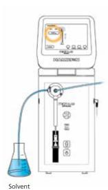
**Step 2.** Trigger the hand probe to fill the left syringe with Solvent.
