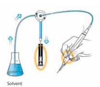
**Step 3.** Trigger the hand probe to dispense the Solvent into a vial.
