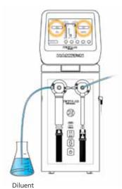
**Step 2.** Trigger the hand probe to fill the left syringe with Diluent and aspirate Sample into the hand probe with the right syringe.
