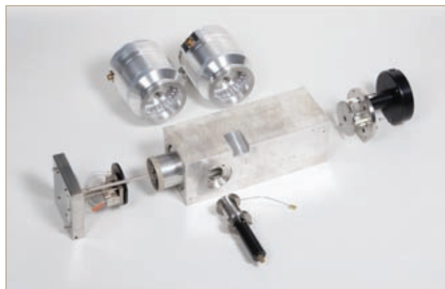
Exploded view of the main MS components
