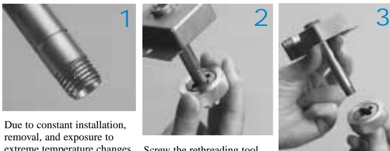
Due to constant installation, removal, and exposure to extreme temperature changes, threads on GC parts easily become worn and damaged. This can cause a poor seal, and oxygen can enter the system, compromising analytical results and possibly destroying expensive analytical columns.
