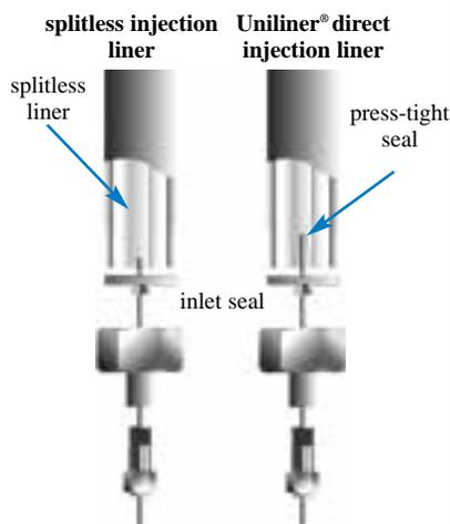
*A Uniliner® direct injection liner prevents the sample from contacting metal surfaces in an injection port, so sample adsorption and catalytic decomposition are reduced and responses for high molecular weight compounds are greater.*
