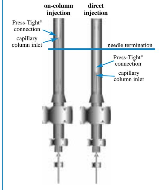
In contrast, a direct injection is made into a 2mm or 4mm ID injection port liner, and the large buffer volume of the liner ensures adequate space for sample vaporization. The vaporized sample is transferred to a 0.32mm or 0.53mm ID column. Larger sample volumes can be used with direct injections, with minimal sample backflash and solvent peak tailing.
