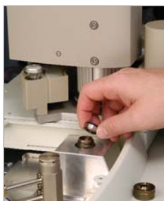
Remove septum cap, septum holder, septum, and septum support.
