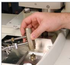
Remove FID cell assembly.
