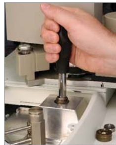
Turn counterclockwise to loosen liner cap.
