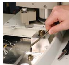
Use tweezers (cat. #20101) to remove jet.
