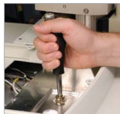
Turn counterclockwise to loosen jet.
