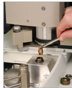
Use tweezers (cat. #20101) to remove liner cap.
