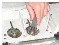
Use the smaller end to remove the septum nut.
