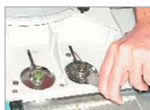
Use the larger end to tighten the split/splitless weldment nut.
