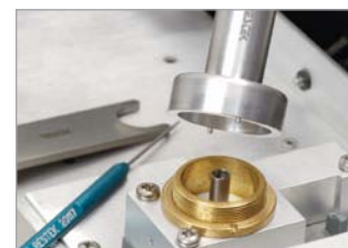
Easily loosen the nut by aligning the two pins on the bottom of the wrench with the two open slots on the nut...
