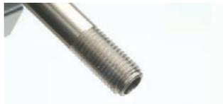
Repeated installation, removal, and temperature changes cause wear and damage to threads on GC parts. This can cause a poor seal, and oxygen can enter the system, compromising analytical results and possibly destroying expensive analytical columns.
