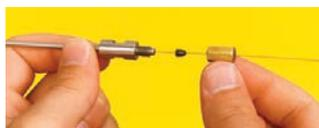
Install the nut and ferrule onto the column, then insert the column through the installation tool, exposing several centimeters at the exit end. Tighten the nut (not depicted).
