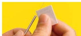
Score and remove the exposed end of the column.
