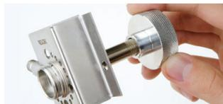
Simply screw the rethreading tool onto the part, unscrew, and inspect the threads. Repeat as necessary. When done, wipe threads clean with methanol to remove any debris.
