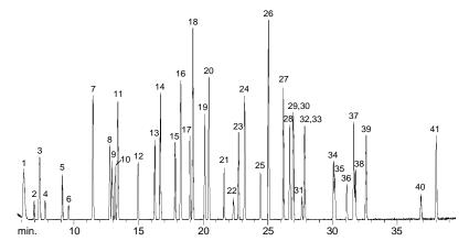
60m, 0.32mm ID, 3.0µm Rtx®-1 (cat.# 10187). 5mL of 2ppmv TO-14 standard. Oven temp.: 30°C (hold 4 min.) to 250°C @ 7°C/min. (hold 15 min.); Detector: MS; Det. temp.: 250°C; Carrier gas: helium; Linear velocity: 21cm/sec. set @ 30°C; Ionization: El; Scan range: 34-280 AMU; Preconcentrator conditions: Nutech 3550 A Preconcentrator; Cryotrap temp.: -160°C; Cryotrap desorb temp.: 150°C; Cryofocusing unit temp.: -190°C; Cryofocusing desorb temp.: 150°C.
