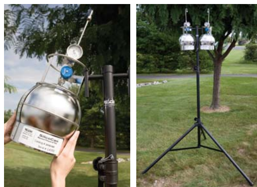
Air Canister Tripod conveniently holds 2 air canisters.
