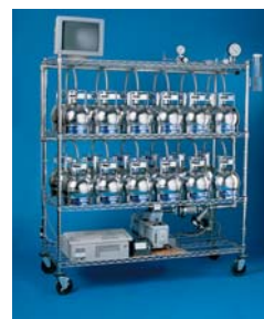
Figure 10 User-designed system for cleaning 24 six-liter canisters.
