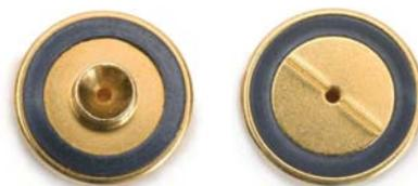
**Figure 2** The Dual Vespel® Ring inlet seal achieves a lower leak rate at lower torque than the conventional metal inlet seal at 200°C.
