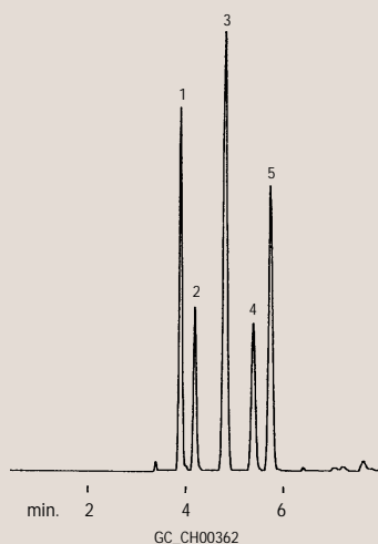
Figure 6 Reactive chlorosilanes analyzed using a 60m Rtx®-200 Column.
