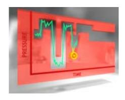
ning caused by blockage, leakage, air bubbles, needle damage, valve problems, etc can be easily recognized in case of suspected erroneous results. The injection pressure profile ("pneumogram") can be linked to assay reports for easy verification afterwards.
