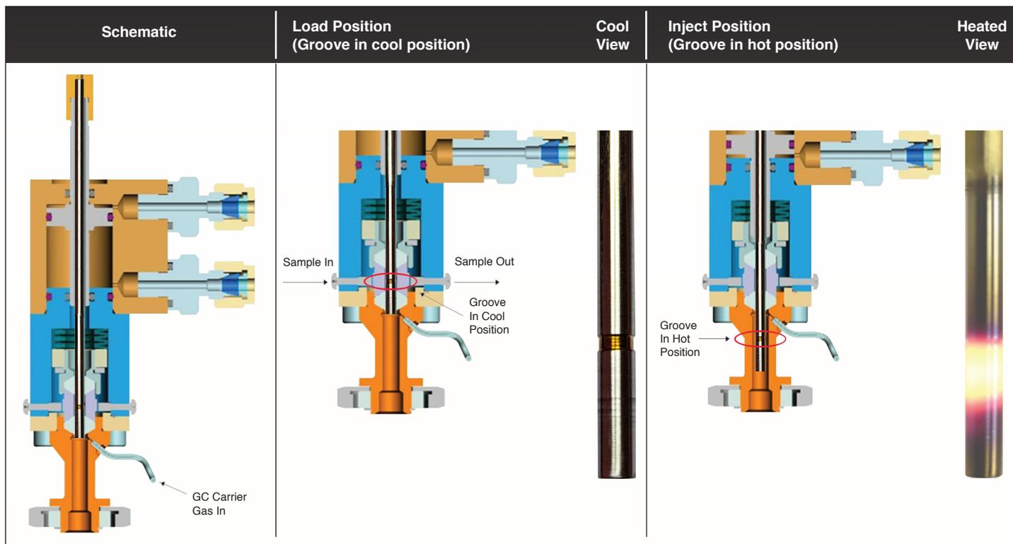
The HPLIS® is unique in that the sample components are maintained at a temperature and pressure level that allows them to remain intact until analysis, at which time they are flash vaporized and introduced directly to the head of the GC column.
