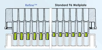
Extended tip length when compared to standard wellplate depth minimizing the risk of inter-well crossspray
